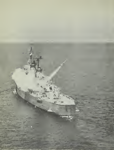
VERSATILE MK 46-0 torpedo can be launched from fixed wing aircraft (right), Asroc tubes as shown in USS Norfolk test launching (left), helicopters, and surface ship torpedo tubes. Torpedo is scheduled for Fleet in summer.
